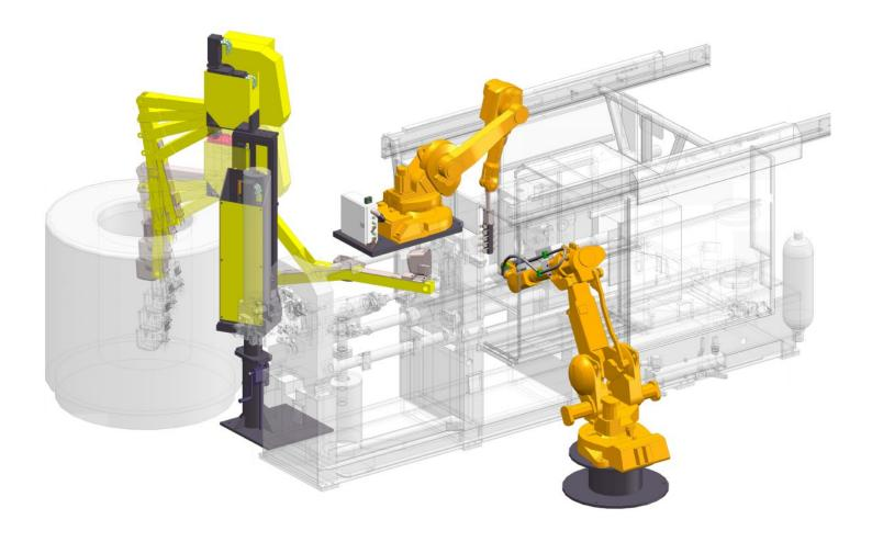
Pomac Automation has got more than 30 years of experience in cell integration. The ladlers, sprayers and robots are installed on all types and sizes of die casting- and gravity machines.
