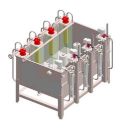
The cooling basin is ideally suitable to cool down the cast part immediately after die casting. The two metal filters, which can quickly be cleaned when needed, are operated in the change time. The basin is cooled by a tube heat exchanger, which is attached to the cooling system of the foundry and a circulation pump. A metal filter prevents glitter and casting remainders entering the circulation pump. This concept is a simple and economic solution and supports full cell automation.
